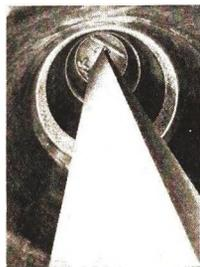
A belt of paper carries static electricity to the top of the generator.
